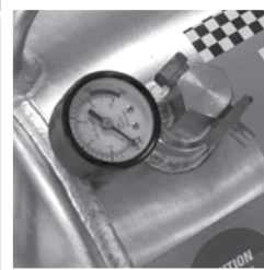
Built-in pressure gauge shows tank pressure
